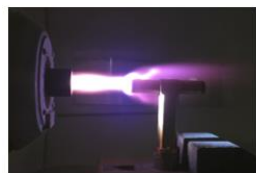
IRS PWK4 Air, 3 kPa, ~6 MW/m 2
