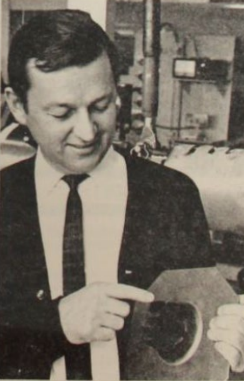
Dr Stalker examining a metal diaphragm blown out in a wind tunnel experiment. The diaphragm is mild steel, quarter of
